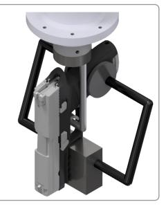
break. The maximum force required to pull the trigger and fire the handgun should be 5.5lb, +/-0.5lb. Additionally, the spring-actuated trigger reset should be less forceful while still remaining tactile enough to allow the user to know the trigger has been reset and is ready to fire again.
